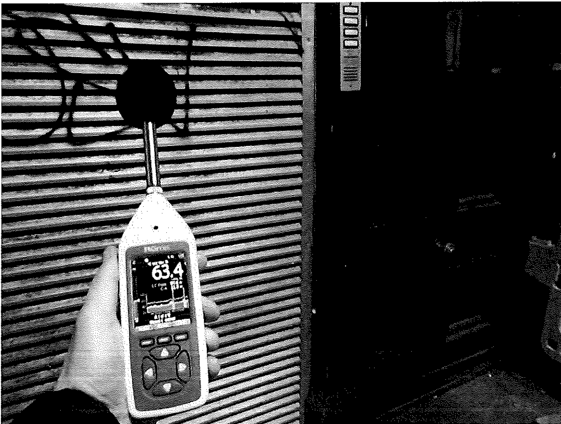
Figure 4: Plant noise at 1m.
